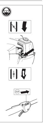
WARNING! When the engine is started with the choke lever in either the choke- or start throttle position the cutting equipment starts to rotate immediately.
